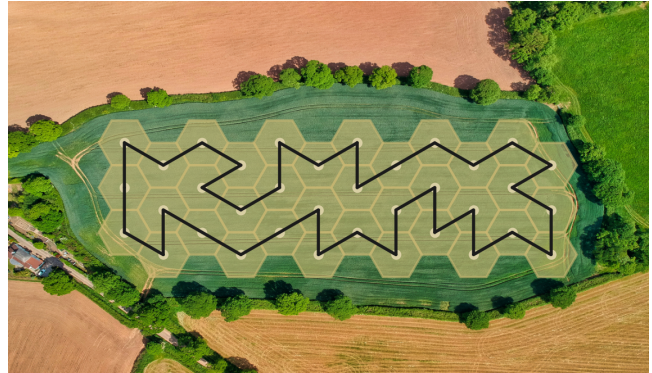
Fig. 1. An example of a solution to the sample placement and shortest tour problem. The vertex set (white circles) of the tour (black) guarantees accurate predictions in the hexagons (yellow), thereby covering the field.
