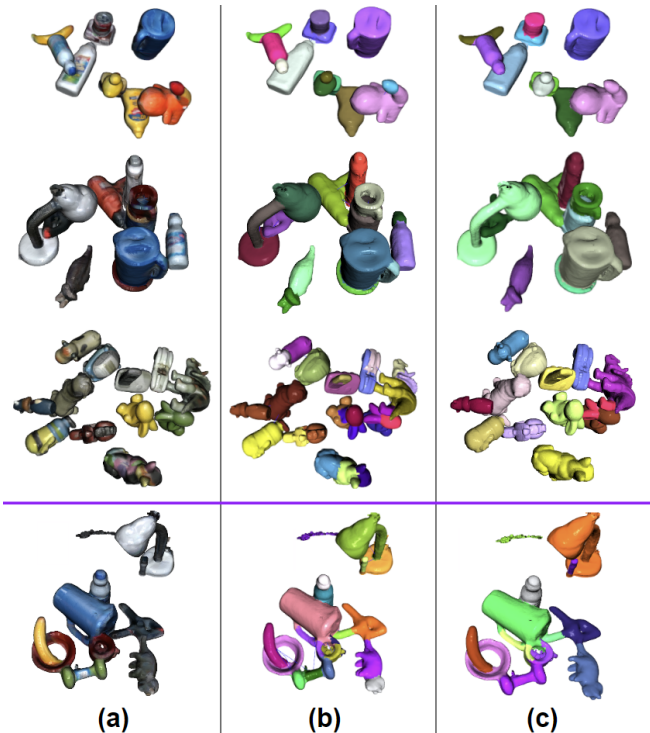
Fig. 6: Intermediate Qualitative 3D Segmentation Results (a) Reconstructed object point clouds in their original color. (b) Segmentation results from LCCP + SymSeg. (c) Object pseudo labels after graph matching and pruning given over-segmentation results as inputs. A failure case of over-segmentation is shown in the last row, where part of the “pitcher” and “cup” are not separated and the “cup” is segmented into inconsistent pieces. This cannot be addressed during graph matching.
