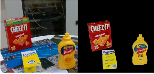
Fig. 2. Object configuration that was used for sequence 4 (left) and object poses as estimated by PoET (right). Note the difference in object package coloring between real-world objects (left) and YCB-V objects used for training PoET (right). The left image, as shown here, is directly fed into our pose estimation framework to get the 6-DoF relative pose measurements.
