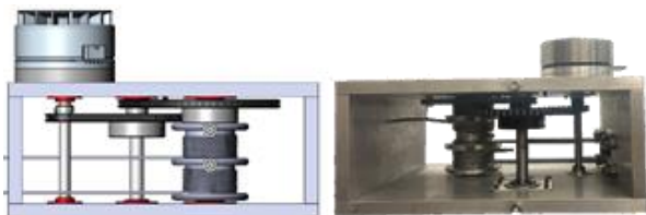
Fig. 1. A CAD model (left) of one of the two off-board actuation systems and photo of the fabricated equivalent (right).
