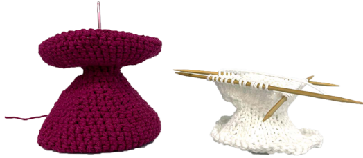
Fig. 2. A crochet object (left) and a knitted object (right) which carries the same properties as imitation-crochet warp knitting. Both objects use the same pattern, hook and needle size, and type of yarn. The crochet object holds its three-dimensional form better than the knitted object, which is more malleable.
