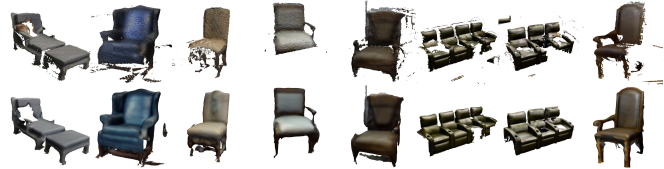
Fig. 4. Objects reconstructed using the proposed method [Top] and their corresponding ground-truth meshes [Bottom]. Notice some artefacts due to erroneous segmentation masks.
