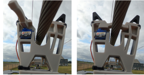
Fig. 9: Left: Primary gripper in open position. Right: Primary gripper in closed position supporting the UAV.
