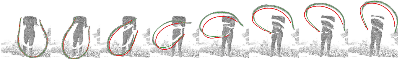
Fig. 5. DLOFTBs (green) and CDCPD2 algorithm (red) on real-data 3D cable tracking sequence. With the fast movement of the cable and insufficiently large cable model updates, CDCPD2 could not track the moving cable. In contrast, our approach accurately tracks the cable shape throughout the sequence.
