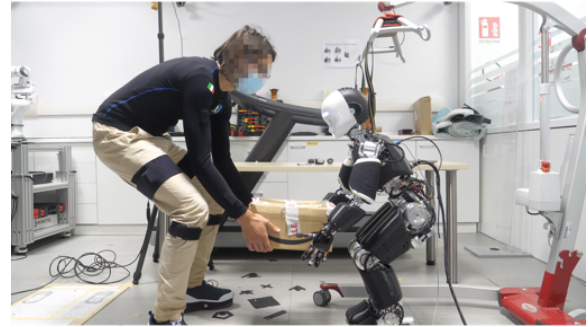
Fig. 1: Human-robot collaborative scenario where an iCub humanoid robot and a sensorized human lift a payload.
