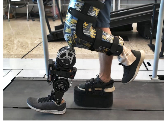
Fig. 2. Experimental setup showing an able-bodied subject using the powered knee-ankle prosthesis with a leg-bypass adapter.
