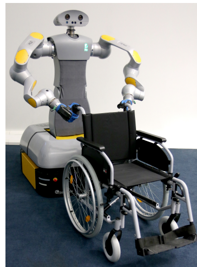
Fig. 1: HoLLiE coupled to a wheelchair.
