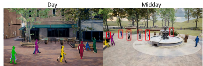
Fig. 6: Example of qualitative results with the tracker PHALP. Left: results on Day data. Right: results on Midday data. The failures (missed people) are highlighted with red bounding boxes. In this case, correspond with people with low resolution.
