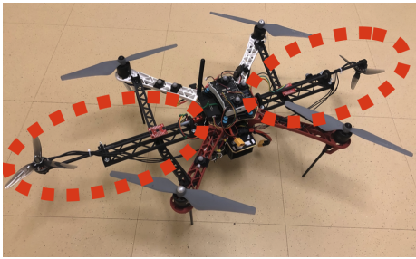
Fig. 3: Two-arm haptic suit prototype (marked using dashed lines) mounted on a DJI Flamewheel F450 drone [28].
