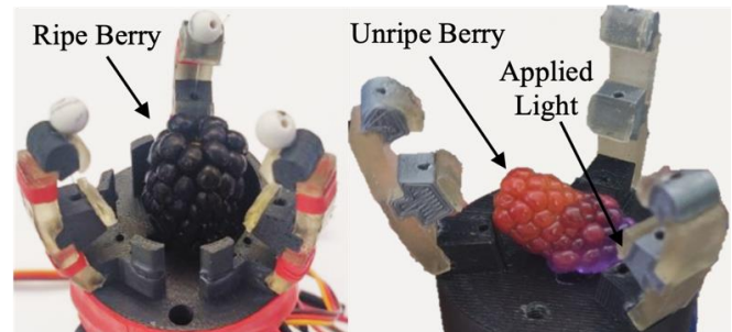
Fig. 5. Left side shows reflectance detection procedure for ripe blackberry and right side shows unripe blackberry being tested. Note that the ripeness sensor composed of LEDs and a photodiode are integrated into the palm of the shown gripper.
