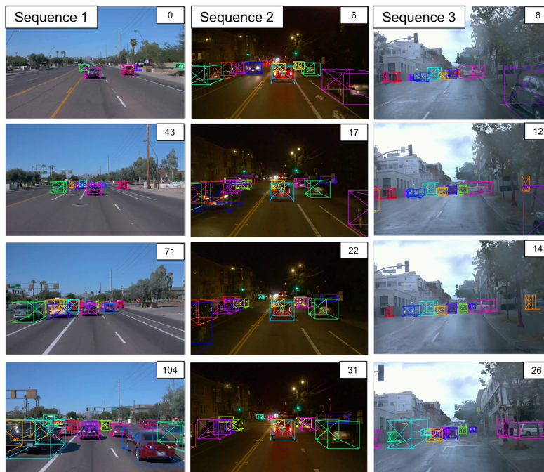
Fig. 3: Qualitative results of our model on diverse video sequences from Waymo dataset. Sequence 1 has long tracks. Sequence 2 has poor lighting conditions. Sequence 3 has adverse weather. Tracking is performed using LiDAR point clouds. The RGB images are for illustration only.
