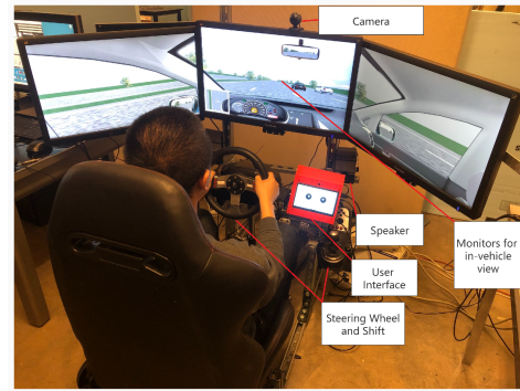
Fig. 1: The cooperative driving simulation testbed.
