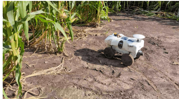
Fig. 1: We present a solution to autonomously navigate in farm environments. By fusing multiple sensors, our system is able to smartly switch between reference modalities to provide safe navigation in real agricultural scenarios.
