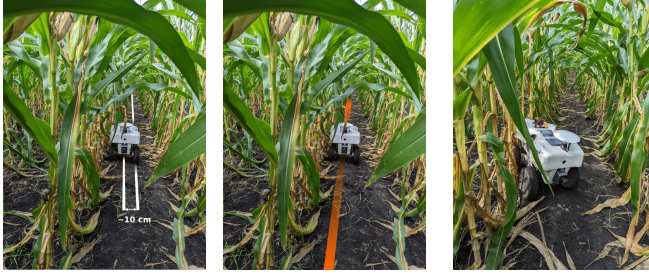
Fig. 8: Navigation offset generated by low GNSS reliability. Due to multi-path, even RTK severely suffers under canopy, causing (from left to right) A) The robot navigates with a constant offset; B) The reference path shifts to the left; C) A failure mode that was frequently observed in the GNSS-only navigation due to the shifted reference path.
