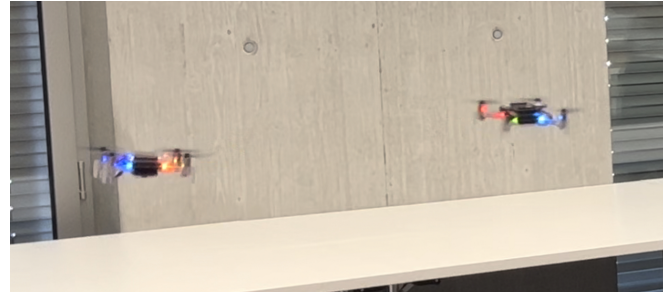
Fig. 1. Our in-field system: nano-drones' relative visual pose estimation.
