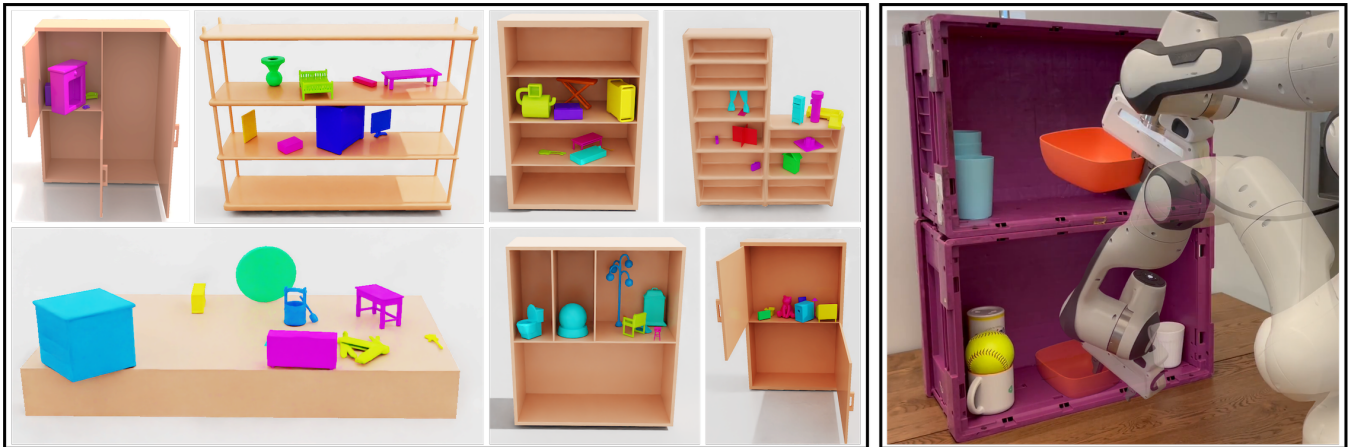
Fig. 1: CabiNet is able to ( right ) perform complex rearrangement tasks in novel, cluttered scenes on the real robot from just partial point cloud observations without object or environment models. The model is trained with over 650K procedurally generated synthetic scenes ( left ).
