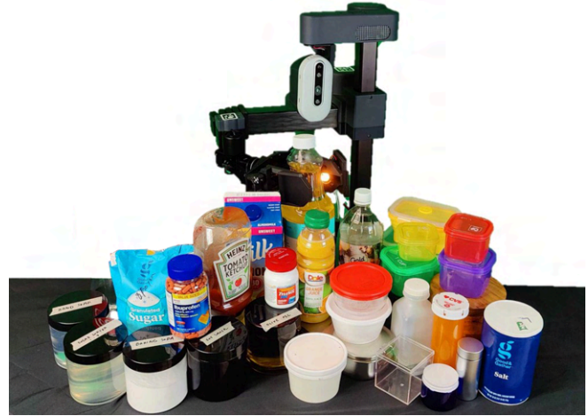
Fig. 1: SLURP gripper mounted on a mobile manipulator (Stretch RE1), surrounded by a variety of containers and contents that the novel system can identify without touch.
