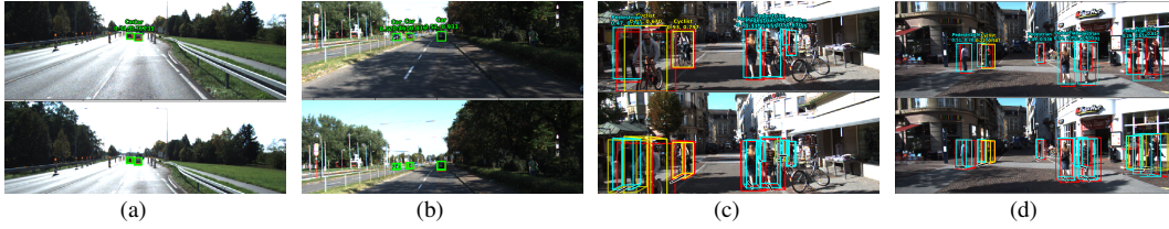
Fig. 4. Visualizations of results on the KITTI validation set (Please zoom in to see better). The upper part is the 2D detection box with detection IoU (right) and classification score (left); the lower part is the 3D detection box. red: The ground-truth boxes, green: The car detection boxes, blue: the pedestrian detection box, yellow: the cyclist detection box.
