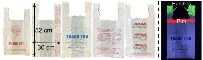
Fig. 3: Left: 5 plastic bags. The first 4 are used to train the perception module (Sec. IV-A). Bags 1 and 5 (test bag) are used in experiments (Sec. V). Right: Bag 3 painted with green UV paint on its handles and red UV paint around its rim, under UV lighting.
