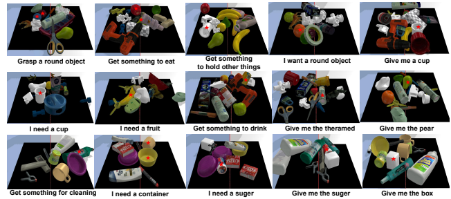
Fig. 3. Test cases in simulation. The top two rows demonstrate the arrangements with seen objects, while the bottom row shows the arrangements with unseen objects. The target objects are labeled with stars.
