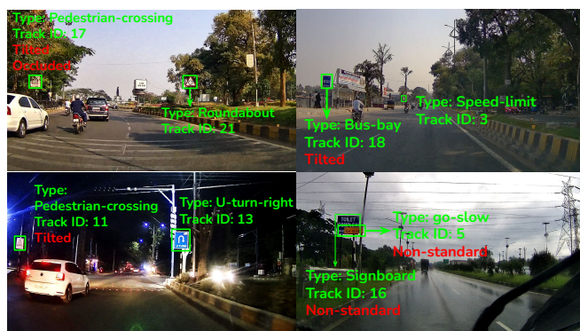
Fig. 3: Annotated frames from MTSVD exhibiting frames having signs with their relevant cues. Top (left to right): a roundabout with pedestrian-crossing, bus-bay with speed-limit. Bottom (left to right): u-turn-right with pedestrian-crossing (night scene), go-slow and Signboard (rainy weather).
