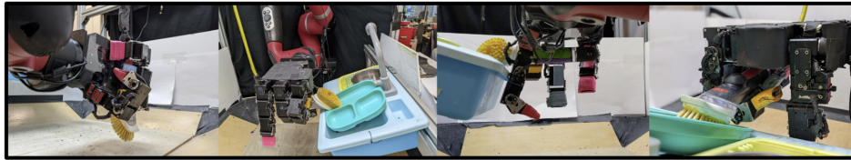
Fig. 1: Filmstrip of the final learned brush skill. Our agent is able to learn to grasp, in-hand reorient, and brush a surface using a kitchen brush. After around \sim 18 hours of unattended learning, our system successfully performs each of these sub-tasks with \geq 80\% success.
