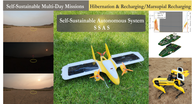
Fig. 1: Indicative instances of the hybrid micro aerial Self-Sustained Autonomous System (SSAS), capable of solar – and externally supplied– power harvesting, as well as hyper-efficient recharging relying on full systems hibernation.
