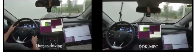
Fig. 5. Experiment video screenshot. The left picture shows the reference trajectory collected by the human driver, while the right picture shows the synchronicity of DDK-MPC for tracking the reference trajectory.
