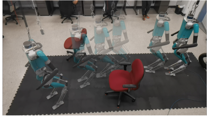
Fig. 1. The snapshots of the bipedal robot, Digit, following the collision-free path generated by the proposed algorithm.
