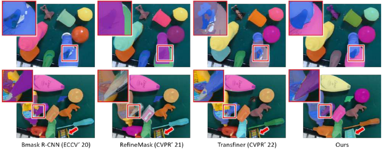
Fig. 6. Comparing instance segmentation results with the SOTA methods on the GraspNet. We emphasize the cluttered regions in red boxes. Our method generates precise masks with clean and sharp boundaries for these regions, whereas other methods fail to accurately distinguish the nearby instances.
