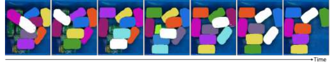
Fig. 10. A picking sequence according to our mask selection strategy, where the object(s) painted white has the highest boundary IoU value.
