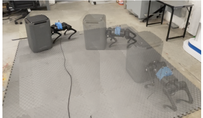
Fig. 1: Motion snapshots of Unitree A1 robot manipulating a 5 kg object to follow a circular trajectory. Supplemental video: https://youtu.be/amzgE4-Yrig
