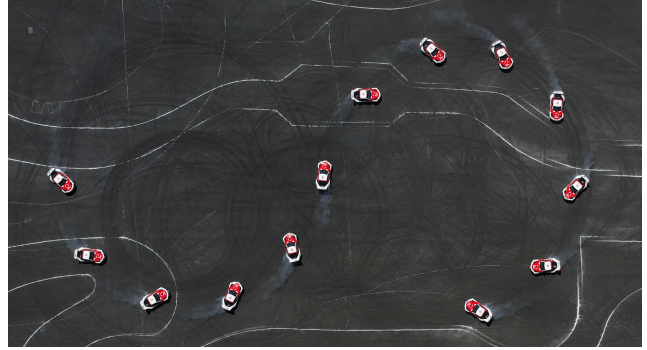
Fig. 1. A photocomposite showing stills from an overhead drone video of a fully autonomous experiment superimposed at 1s intervals.
