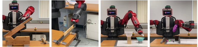
Fig. 1: TYPICAL COMPLEX MANIPULATION TASKS: (From left to right) Manipulation of object constrained by a revolute joint; Manipulation of object constrained by a prismatic joint; Scooping and pouring; Arranging dishes in a dish rack.
