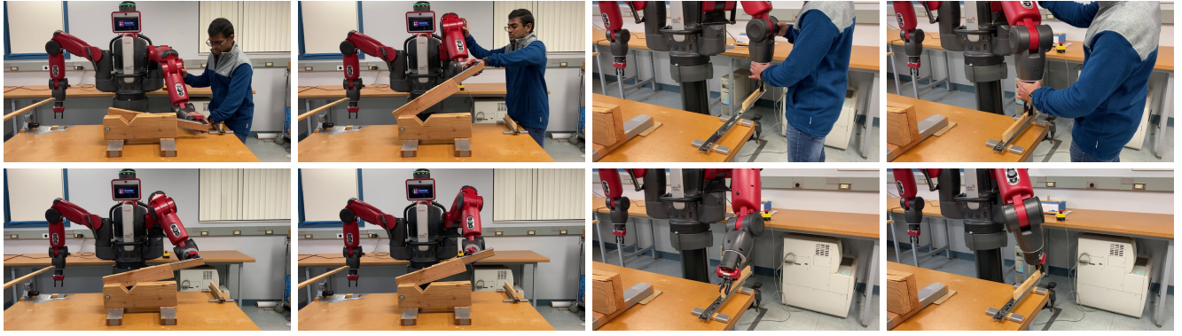
Fig. 2: MANIPULATION OF ARTICULATED OBJECTS: User Provided Kinesthetic Demonstration (Row 1 from Left to Right) : Revolute Joint Demo #3 Start Pose (Revolute Joint Closed Position), Revolute Joint Demo #3 End Pose (Revolute Joint Open Position), Prismatic Joint Demo #3 Start Pose (Prismatic Joint Open Position), Prismatic Joint Demo #3 End Pose (Prismatic Joint Closed Position); Grasping Pose Changes across Trials (Row 2 from Left to Right) : Changes in position and orientation of how the end-effector grasps the object across conducted Trials when using Demo #3 for Revolute Joint (Image #1 - Trial #2, Image #2 - Trial 4) and when using Demo #3 for Prismatic Joint (Image #3 - Trial #3, Image #4 - Trial #4).
