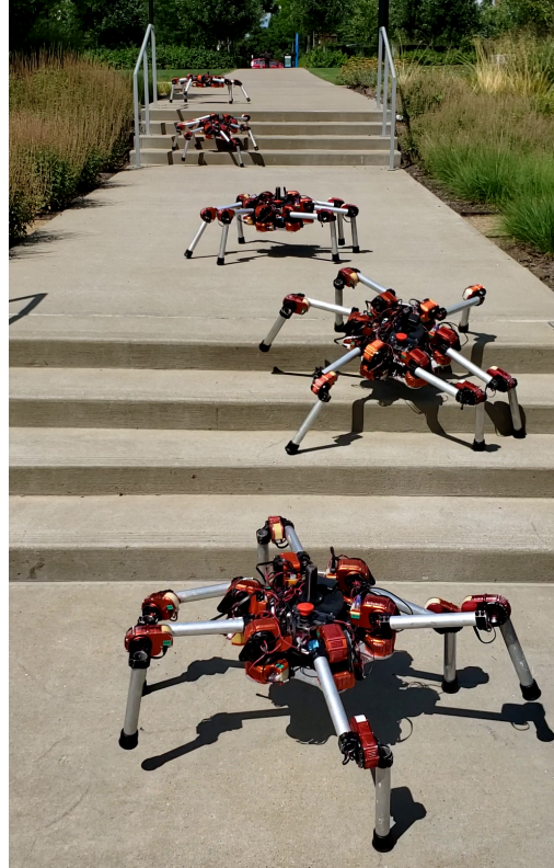
Fig. 1: A time-lapse of our hexapod robot climbing stairs using the onboard vision system and our learned modular visual-motor policy. The steps in the stairs shown here are 14 cm high, which at the robot’s nominal resting stance, is near the distance between the robot body and the ground. A video of this behavior is in the supplementary material and at https://youtu.be/2tCj34zY6kI
