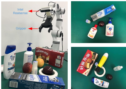
Fig. 5. Real-world robotic grasping experimental setup.
