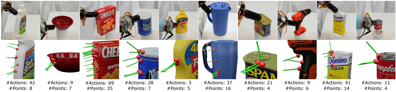
Fig. 5. 10 successful examples of our method in real robot experiments. The top row shows the object poses and the final finger poses. The medium row shows the collected contact positions and normals at termination. The last row shows the results for each trial. Our method reacts to previous observations along the trajectory and gradually moves to the most distinguishable areas for efficient recognition. Each example is accompanied by a real-world video on our project website at https://jxu.ai/tandem3d .
