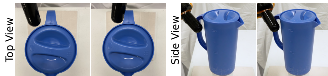
Fig. 3. TANDEM3D angle adjustment move. Our tactile finger with all-around sensing coverage collects a critical contact point on the pitcher handle by adjusting the angle.
