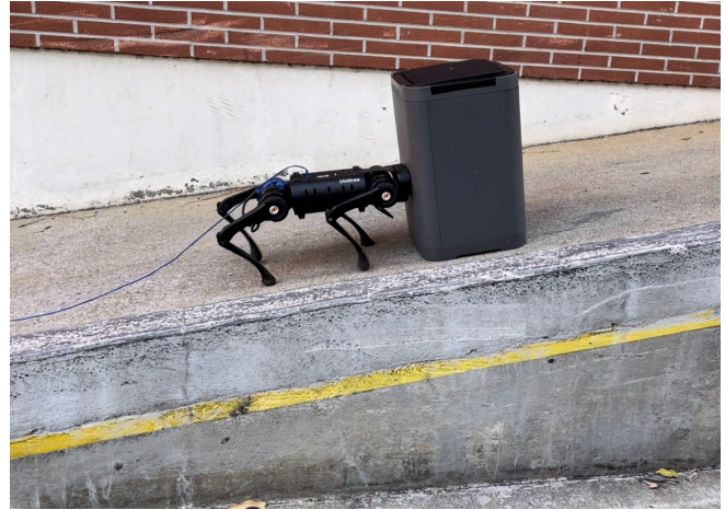
Fig. 1: Unitree A1 robot manipulating an unknown object of 5 kg on an unknown high-sloped terrain. Experimental results: https://youtu.be/-EvSmJRrMFI .
