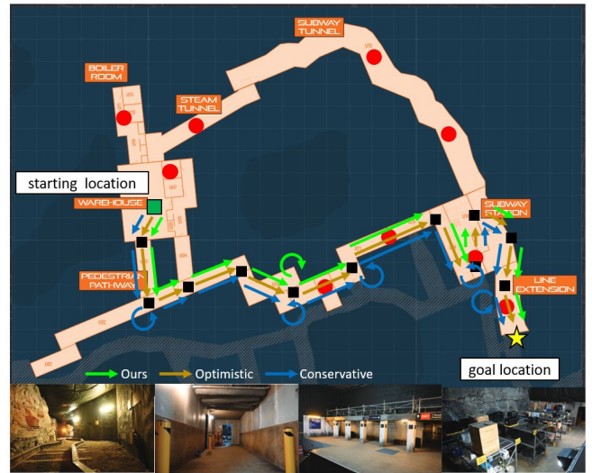
Fig. 4: Course map of the simulation based on real-world urban environment depicted by the photos on the bottom. Red dots on the map marked the location of stairs and rubble. The most likely paths computed by all the methods are overlaid on the map. The circular edges represent information gathering action.
