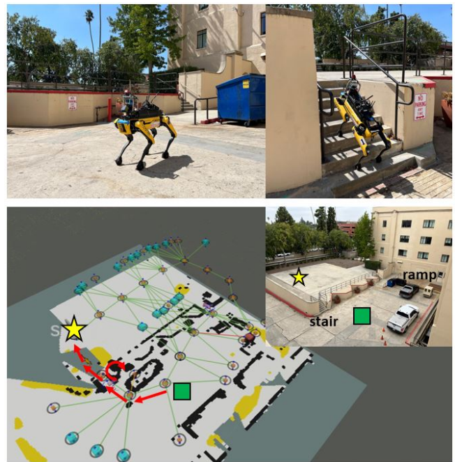
Fig. 6: Top: Field experiment setup in a two-level outdoor environment by using the NASA JPL Spot robot [22] and Spot’s stair climbing behavior. Bottom: Visual representation of the policy computed with the SBG on Information Roadmaps [20]. The red arrows show the most likely path from the starting location (green square) to the goal (yellow star). The circular arrow represents information gathering actions. Initially, the only path in the graph between the starting and goal location is through the ramp. By considering the path through nodes labeled with stairs, the robot chooses a shorter path by climbing the stairs.
