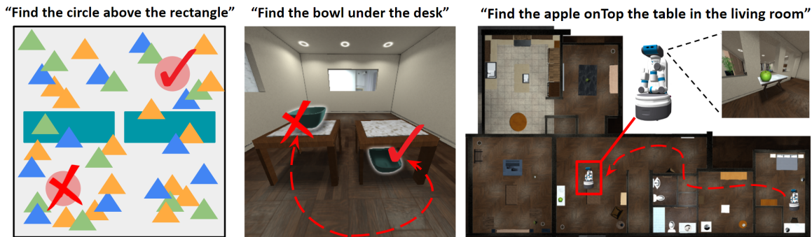
Fig. 2: Three concrete tasks that illustrate relational object reasoning: relational object choice, directed object navigation, and exploratory object navigation. In relational object choice (left), given a relational object goal such as “the circle above the rectangle”, the agent should output a binary choice (left/right) that corresponds to the side of the environment that satisfies the goal. In directed object navigation and exploratory object navigation (middle, right), given a relational object goal such as “the apple on top of the table in the living room”, the agent should output a sequence of discrete navigation actions (forward/backwards/left/right/stop) to find and get close enough to the target object.
