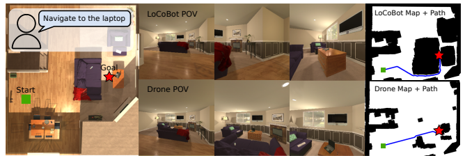
Fig. 5: VLMs enable different embodiments to define their own obstacle maps for navigation. The left image shows the top-down view of an environment. The middle columns show the observations of agents during navigation. The images on the right demonstrate the obstacles maps generated for different embodiments and the corresponding navigation paths.
