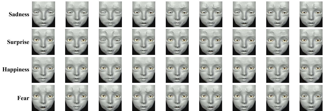
Fig. 4. Solution Matrices of Target Expressions. feature 1 is the vertical coordinates of solution matrices, whereas feature 2 is horizontal. Under the constraints of the target expression and AUs, the solutions are not uniformly distributed in the solution matrices.
