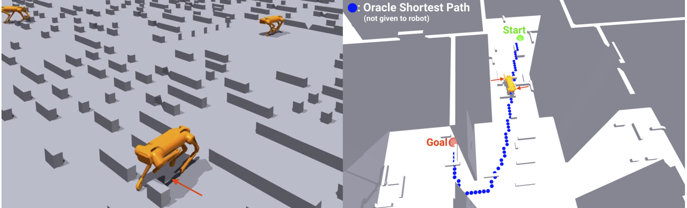
Fig. 1: Left: We learn a visual locomotion policy to follow linear and angular velocity commands while carefully avoiding obstacles with its feet using egocentric depth images. Right: We couple this locomotion policy with a high-level visual navigation policy, enabling AlienGo to navigate to goal locations in novel environments (without a map) while stepping over small obstacles on the ground.
