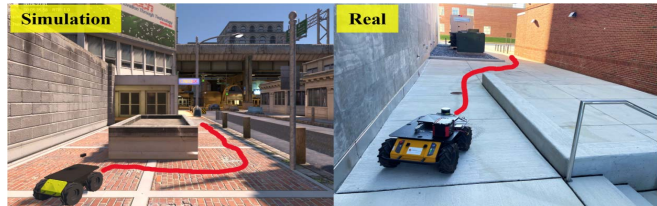
Fig. 5: Trajectories when navigating a Clearpath Husky robot in both simulated and real Urban environments using a policy trained with HT-SPG under sparse reward settings. The trained navigation policy can perform equally well in real world environments.
