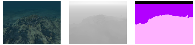
Fig. 3: Dataset instance with RGB image, depth map, and semantic label. is shown in Fig. 5.
