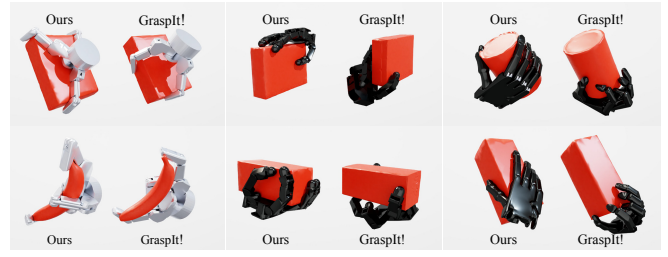
Fig. 4: Contact-rich grasps can be generated by our method which optimizes in the full DOF-space of the hand. The GraspIt! [1] planner mainly generates fingertip grasps. The baseline grasps exhibit fewer contacts that result in reduced stability compared to grasps synthesized by our method.
