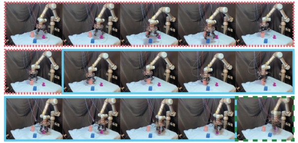
Fig. 4: Film strip depicting phases of real world localization and identification with our pipeline. We see that objects move minimally, while shapes are successfully identified and grasped. Red box shows the localization, blue box shows the interaction, and the green box shows the grasping.
