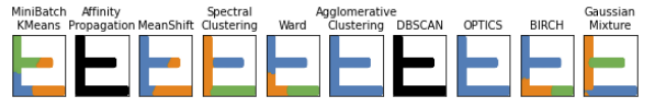
Fig. 1: Clustering methods on a map with three walls. Clustering based on the Gaussian Mixture model leads to a clean separation between the different wall segments.
