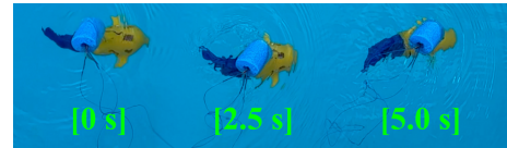
Fig. 11. Overlaid video frames of SunBot swimming in an outdoor pool. The robot is able to reach speeds of up to 0.6 body lengths per second by periodic bending of the tail at 2 Hz with an amplitude of \pm 55^\circ
