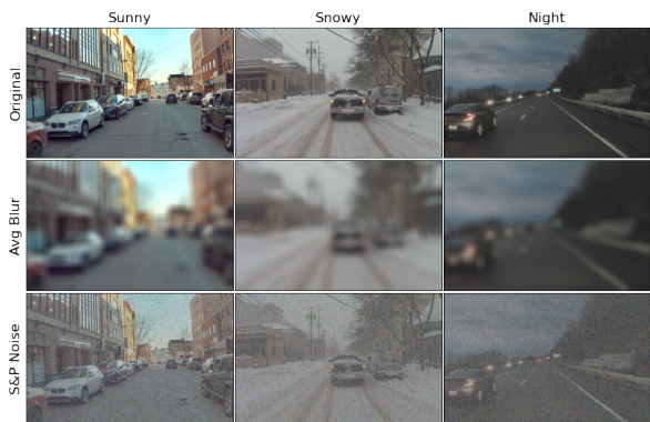
Fig. 7: Examples of corrupted images. Top: original images. Mid: blurred images (average blur with kernel size 80, Bottom: images corrupted with salt and pepper noise (noise amount is 0.5)).
