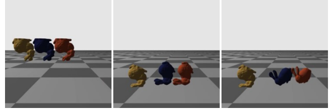
Fig. 3: Comparison between penalty method with damping on dynamics (yellow), proposed method (blue), and position-based Signorini condition (pink). The damping coefficient is chosen to be critically damped with k_n = 1000 , and damping parameter selected as \alpha = 1.5 for proposed method.
