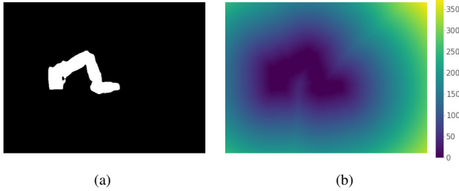
Fig. 4. Visualization of the distance map, with (a) the reference binary mask and (b) the corresponding distance map.
